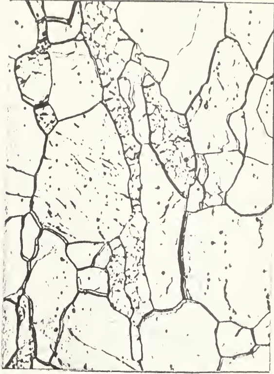
FIG. 25 AT 540°C, UNDER .6%/HR. STRAIN RATE, FOR 30 HOURS (ROCKWELL 30T 40.7)
